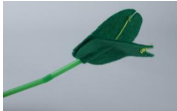
Figure 1. Early prototype made from felt and straw. The felt retracts when two strings are pulled.
